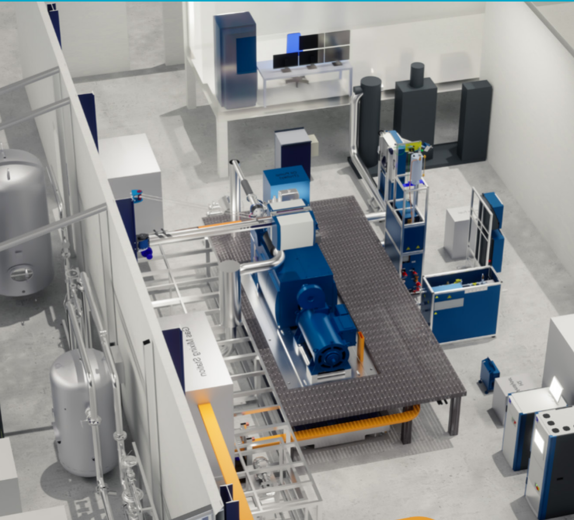
Concept engineering of a Single Cylinder Testbed 230 mm bore for multifuel operation and gas mixing unit (hydrogen, CNG, propane, CO 2 , and ammonia)
